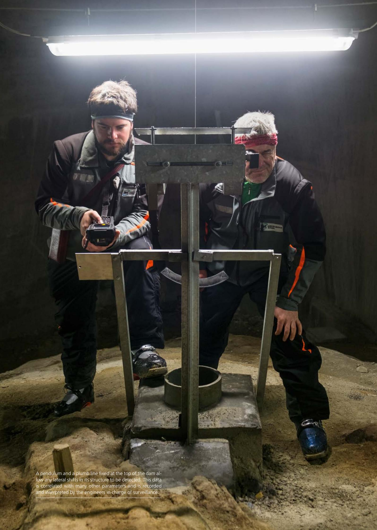
A pendulum and a plumb line fixed at the top of the dam allow any lateral shifts in its structure to be detected. This data is correlated with many other parameters and is recorded and interpreted by the engineers in charge of surveillance.
